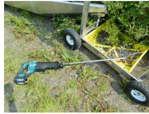
Reciprocating saw with homemade attachment
